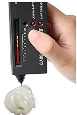
5. After Calibrating, move the instrument onto the jewelry vertically. And stabilize it for 2-3 seconds to obtain the hardness data
