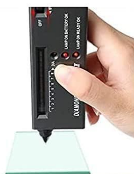
4. Calibrate instrument: contact the probe with glass vertically and turn the switch upward until the indicator light is on at the fifth
