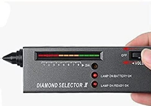
3. After heating, turn left switch until the indicator light is on in the first one
