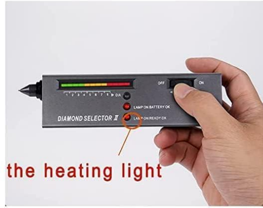
2. Turn right switch to the highest position and wait for the heating light to turn on
