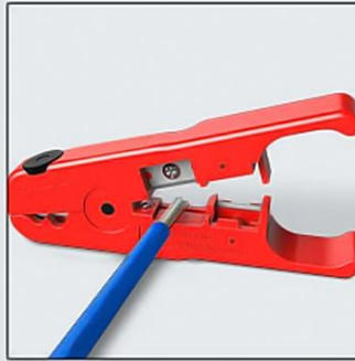
2. Trim all conductor wires
