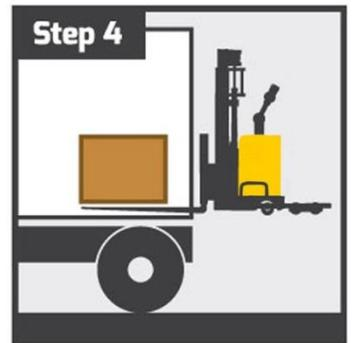
Stacker lifts itself using a reverse lift motor.
